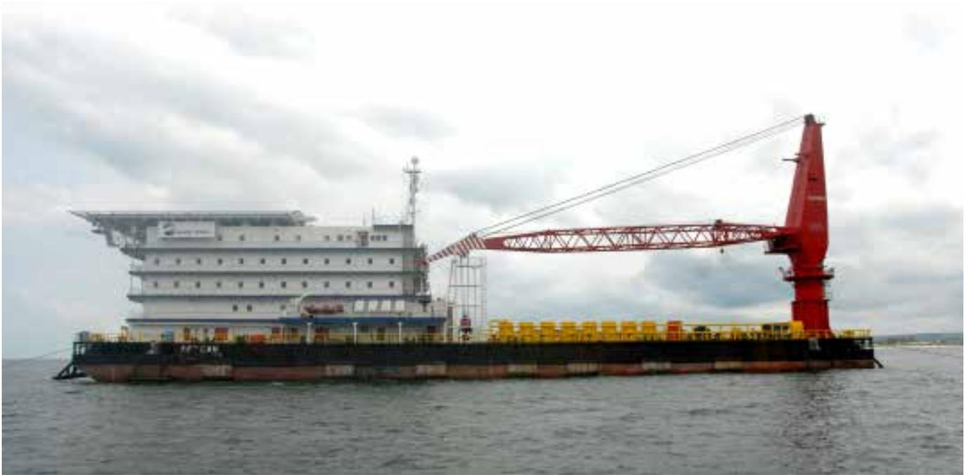
Barge provides support and infrastructure during offshore construction or modification and maintenance. Flat bottom barges are well suited for the calm waters off the coast of many geographies. Can also provide lay-down areas.
